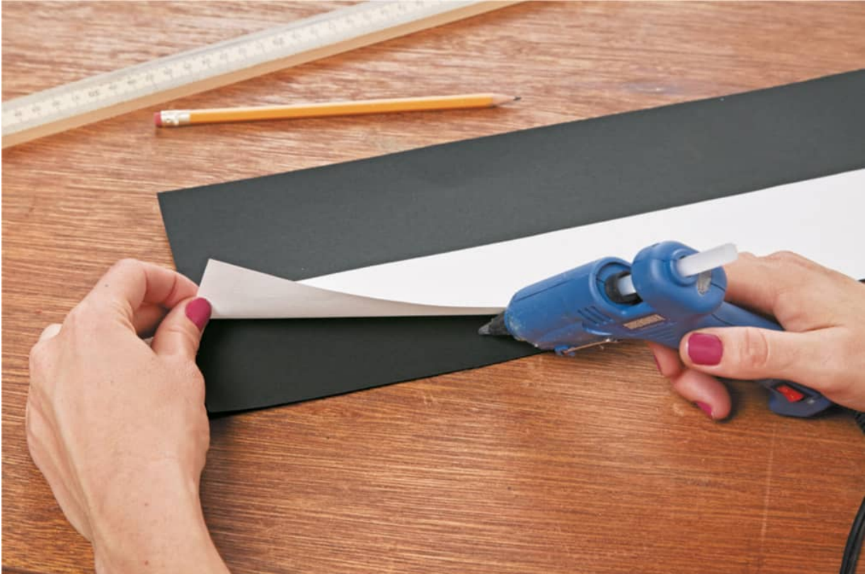
fig. 1. Use a hot glue gun to attach the white paper to the black paper, as these papers are a heavier weight.
