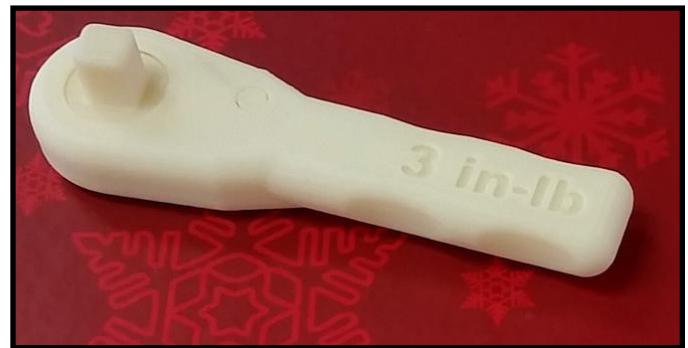
Figure 4.8 - Isometric Projection of 3D Printed Ratchet - Image courtesy of NASA
