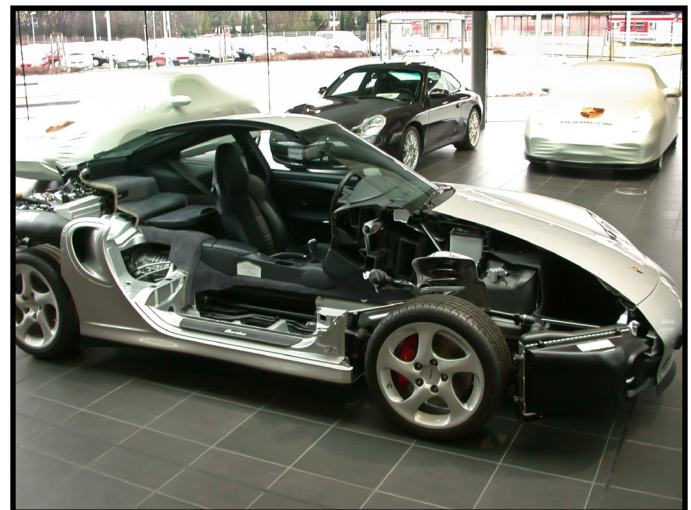
Figure 9.2 - Complex Section View Image courtesy of Maximillian Schoenherr - Wikimedia
